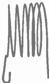
1st speed resistor 6 gauge with 5 turns
