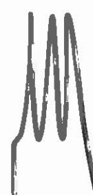
3rd speed resistor 7 gauge with 3 turns
